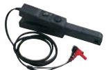
Active AC and DC current probe with voltage output. 2 measuring ranges: 10 A and 80 A Frequency range: DC to 10 kHz Accuracy: error < 2% for currents up to 40 A and frequencies up to 1 kHz Phase error: < 0.5° at 50/60 Hz Length: 230 mm (9.1") Article No.: VEHZ4000
